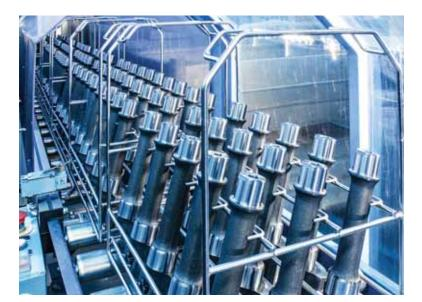
TO MANUFACTURE **ASSEMBLED** CAMSHAFTS, WE USE 'FORCE FREE HEAT SHRINK' PROCESS PATENTED BY EMAG
